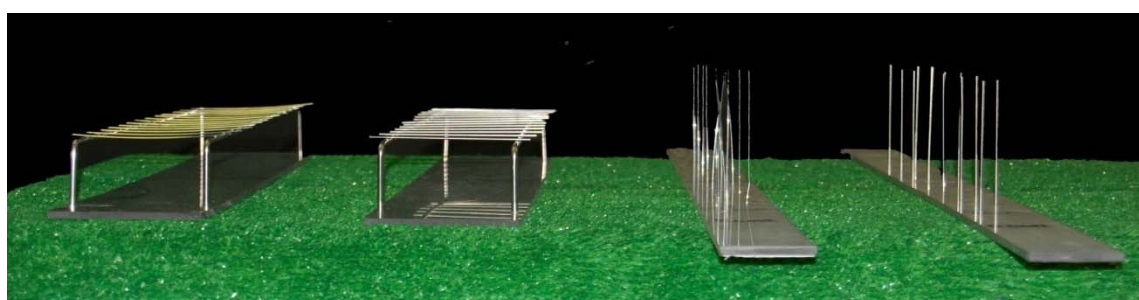
Figure 1. Boom arrangement and target systems used in wind tunnel studies at Silsoe
